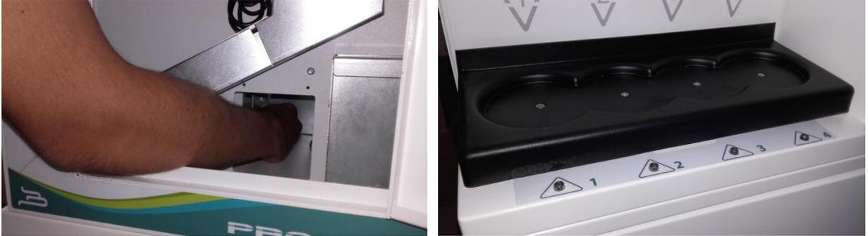
Now open the top trap and the front panel trap. Unscrew the knobs shown in the picture and extract the ducts. It will all come out in one piece. Clean them using just soap and water.
