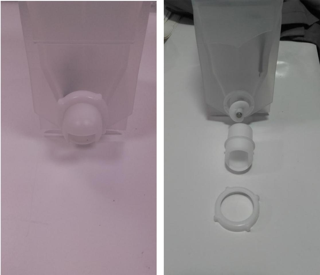
Once you've finished cleaning them, assemble them back again and don't forget to place the nozzle with the opening facing downwards, just as the image shows.
